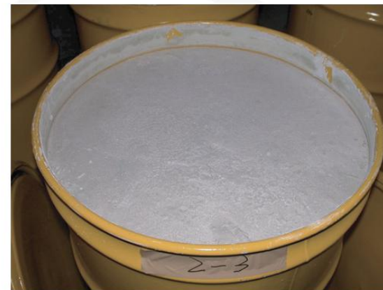
Solidified Object Produced by Pilot Run of the High Volume Reduction Solidification System
